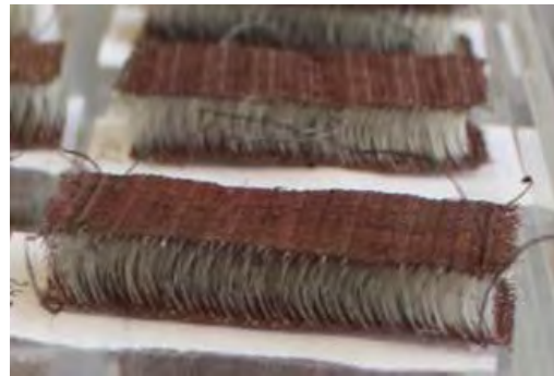
Figure: Wet-chemical ZnO thin film and thermoelectric generators with AZO layers on textiles.
